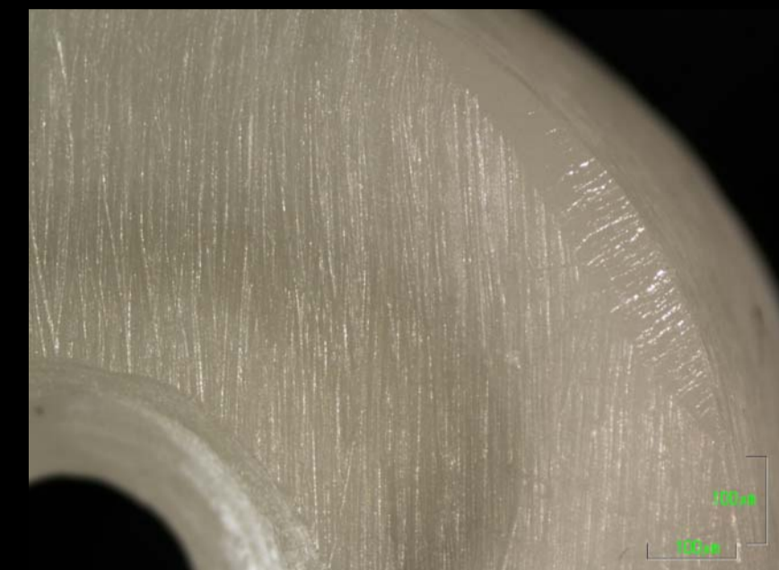
Figure 1: experimentally made bead, fresh state (magnification 10x).
